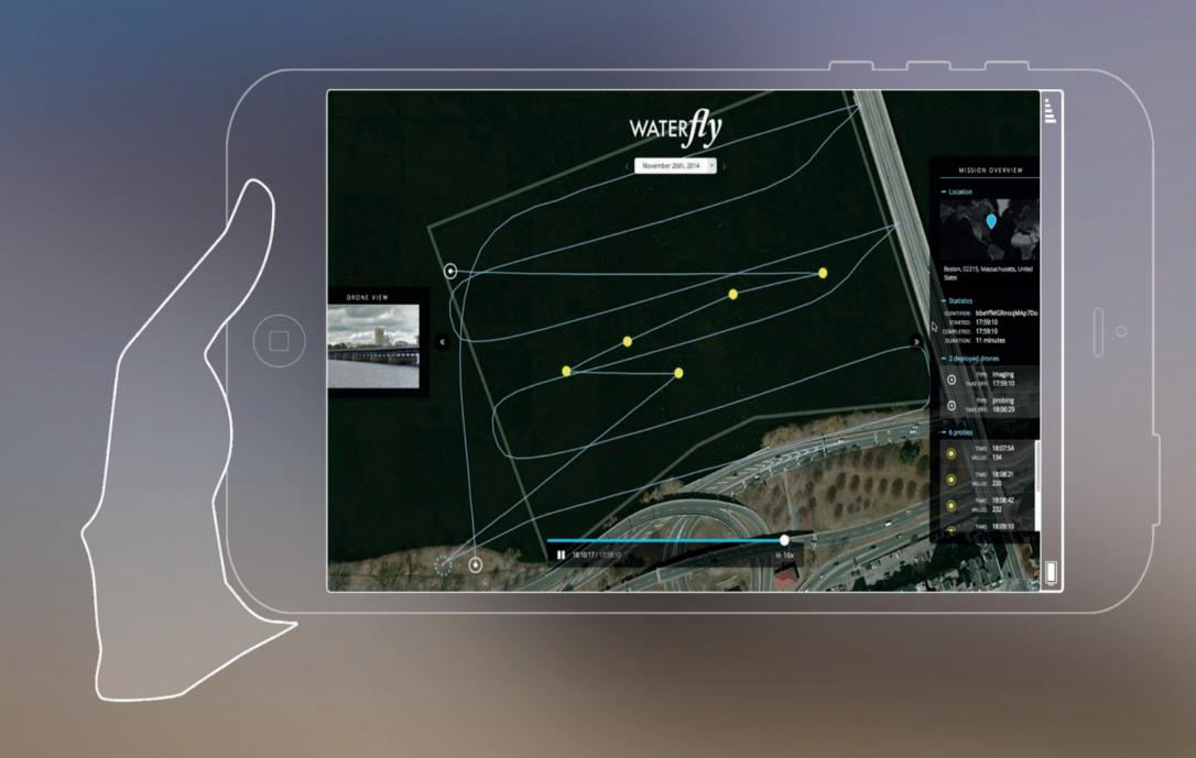
The cloud enabled system combined with real-time computer vision and water sampling for algae detection let the user monitor the mission through the online user interface
